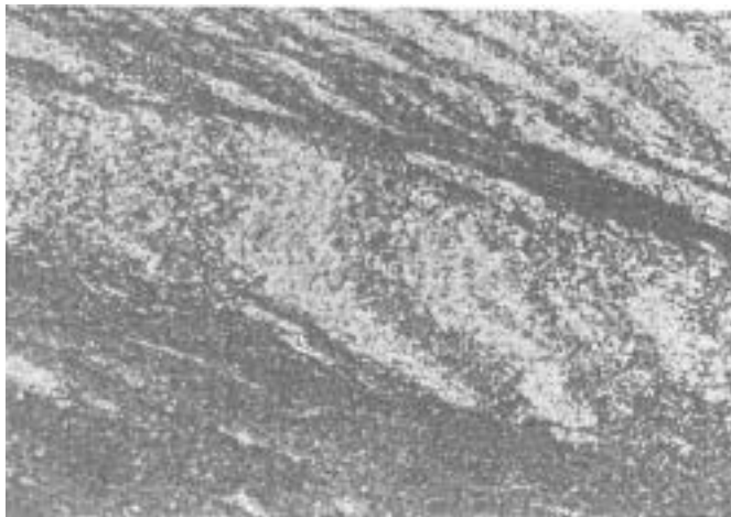
Figure A.6. A cross section of a schist showing almost parallel elongated mica grains (dark grey). The portion shown is about 1 cm from top to bottom.
